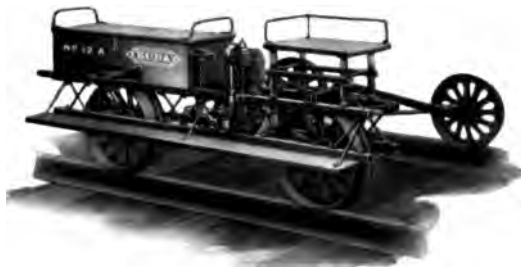
Buda No. 12-A. Inspection Motor Car
